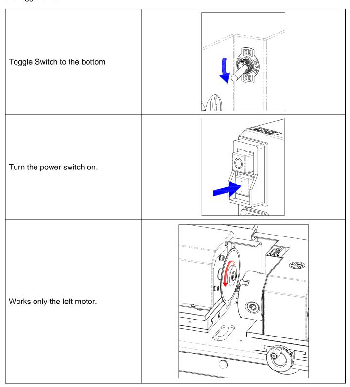
Toggle Switch to the top **X** Please make sure the Spindle locker in the horizontal location. Turn the power switch on. The both sides motors work.
