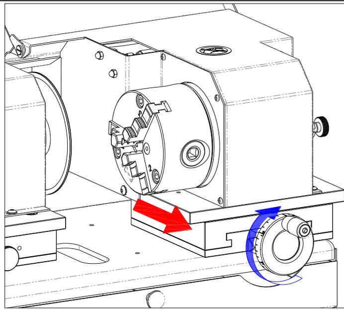
Counterclockwise the Y axis wheel that will move forward the Y axis.
