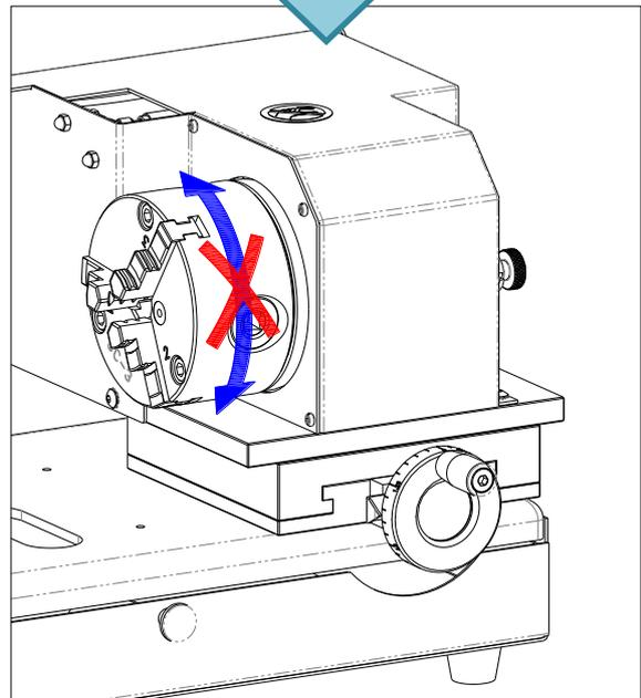
Finishing your job, please keep Spindle locker to horizontal location to avoid motor burned when Toggle switch to the top and others turn on power button.
