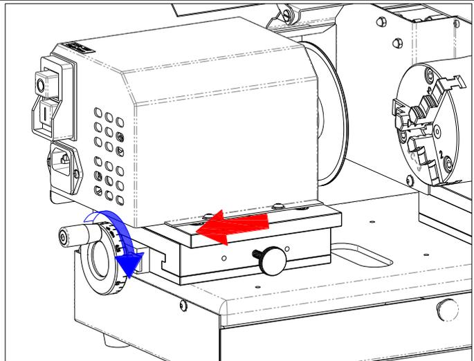
Counterclockwise the X axis wheel moving X axis to the right.
