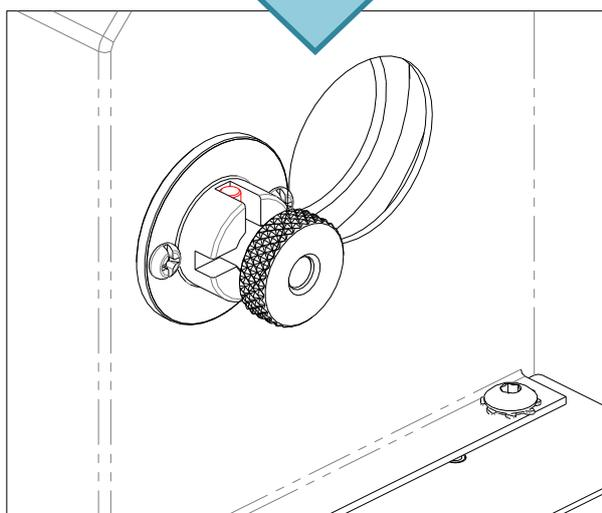
Turn the 3 Jaws spindle and lock on.
