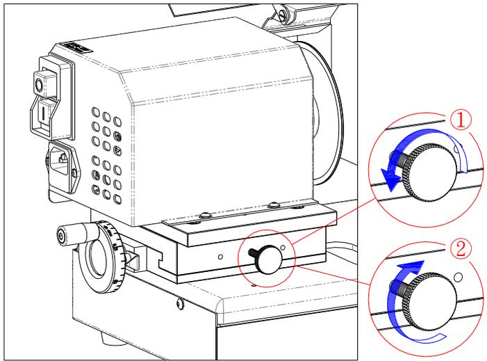
Clockwise the X axis wheel moving X axis to the left.
