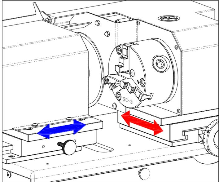
Tighten the X axis Locker.
