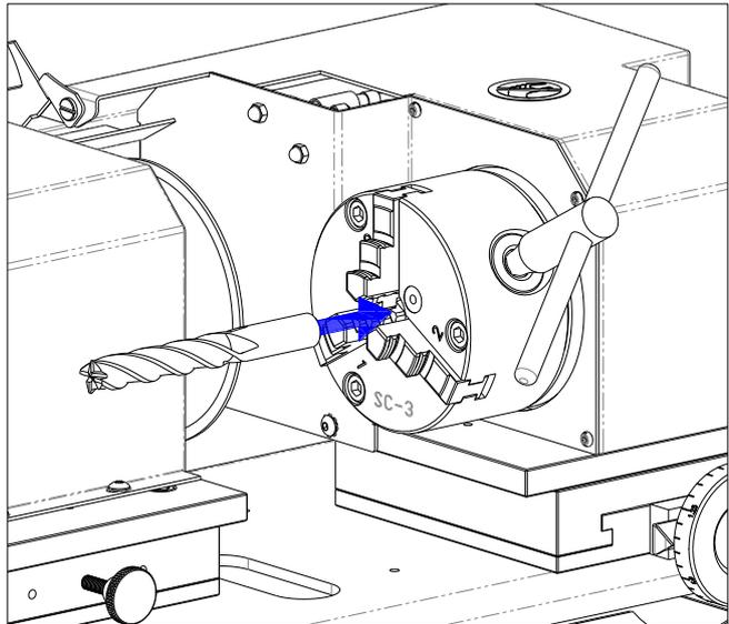
Tighten the spindle
