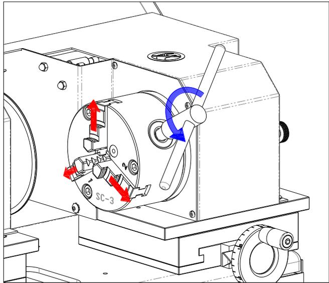
Insert the workpiece.
